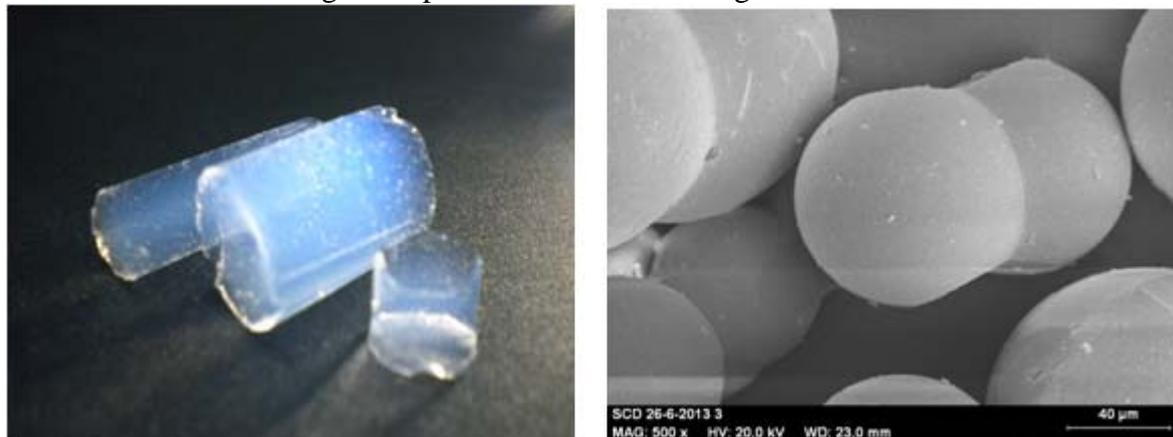
**Figure 2:** Aerogel monolith (left) and aerogel microparticle (right)
